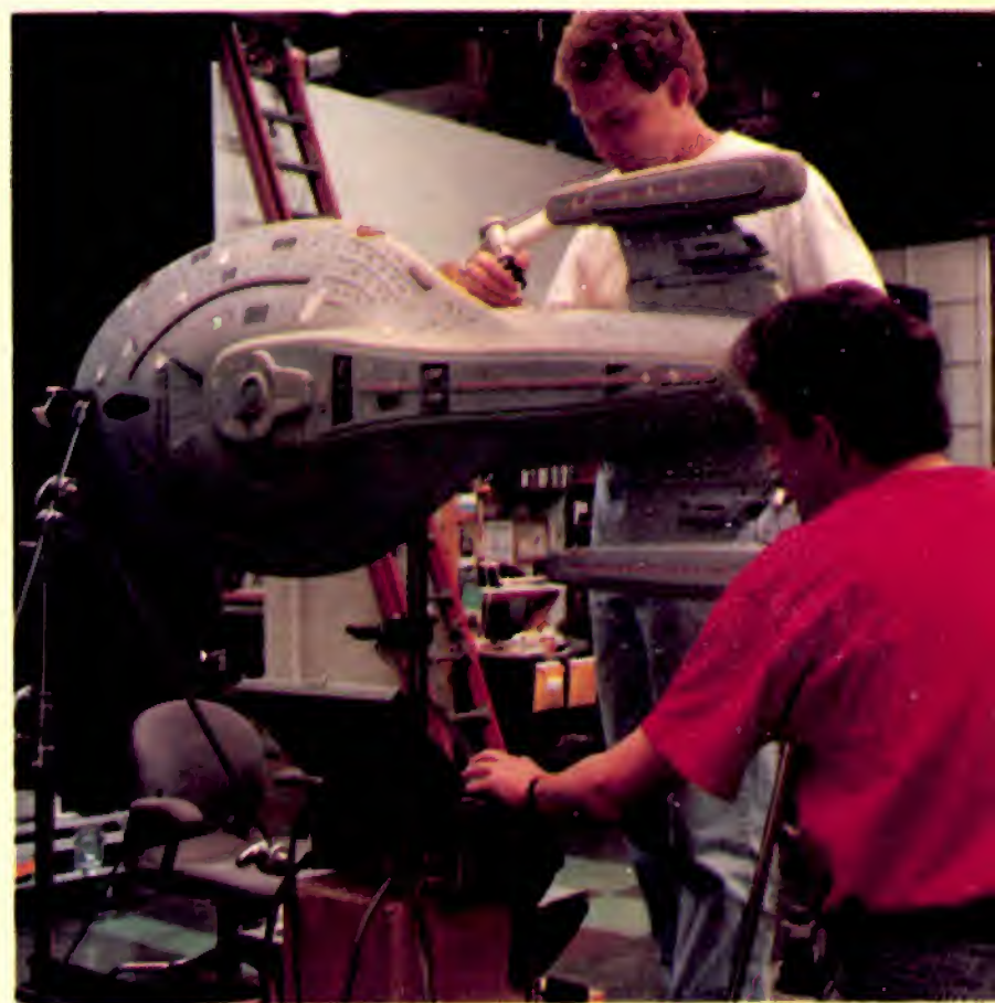
Technicians from Viewpoint Effects of Orem, Utah create the database for a digital version of the Voyager by touching a computer pen to points on a grid on the surface of the model.
